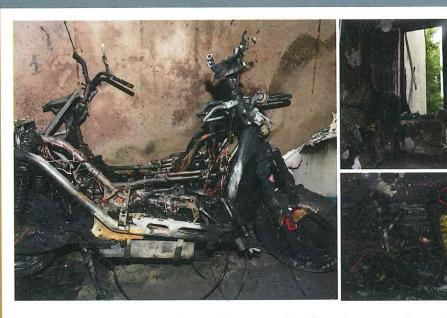
Damaged or unstable batteries and improper charging, storage or disposal can cause the batteries to overheat, leading to an explosive, aggressive fire that spreads rapidly, can reignite and is challenging to extinguish.
